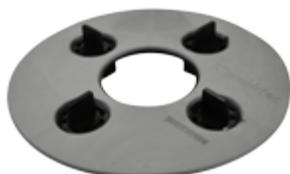
The Uptec SUPA2 accessory, designed to create 2 mm (5/64") joints, is made of two-component material: polypropylene for the fins and rubber to ensure an anti-noise and anti-slip characteristic. The tabs can be removed using the SUPAK key depending on the floor configuration.
